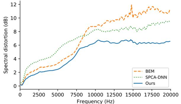
**Fig. 3:** Average spectral distortions for BEM, SPCA-DNN, and our method. The average SD across all subjects and frequencies are 7.23 dB, 6.89 dB, 4.80 dB for BEM, SPCA-DNN, and our method, respectively.
