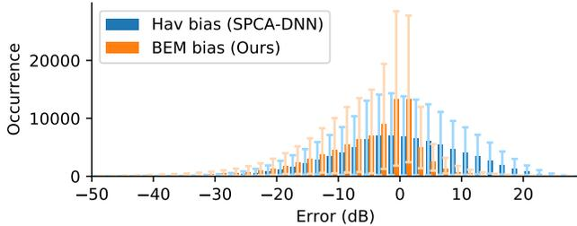
**Fig. 2:** Histogram of errors ( $E$ ) introduced by different biases (blue:  $E_{\text{hav}}$ ; orange:  $E_{\text{bem}}$ ). The histogram is averaged over all 58 subjects in our dataset; the error bars shown in thin lines represent 25 and 75 percentiles of every error bin.
