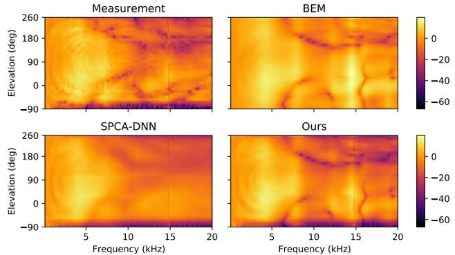
**Fig. 4:** Comparison of measured HRTF in decibels on the median plane with the reconstructed HRTFs from BEM, SPCA-DNN, and ours.
