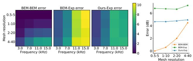
**Fig. 5:** Convergence analysis. BEM-BEM: BEM errors against the finest BEM resolution; BEM-Exp: BEM errors against measurement; Ours-Exp: errors of our method against measurement. Line plot on the right shows the same errors average over frequencies.
