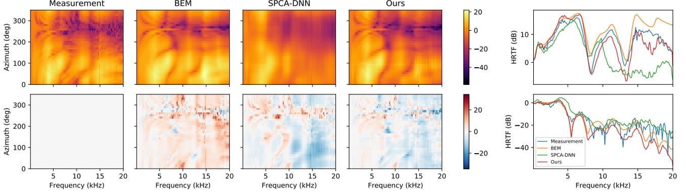
**Fig. 1:** Comparison of measured HRTF on the horizontal plane (0 degree elevation angle) with the reconstructed HRTFs from BEM, SPCA-DNN, and our method. Left Top: HRTFs in decibels; Left Bottom: residual differences between the reconstructed HRTFs and measurement. Right Top: frequency-dependent HRTF at 90 degree azimuthal angle (ipsilateral); Right Bottom: frequency-dependent HRTF at 270 degree azimuthal angle (contralateral).
